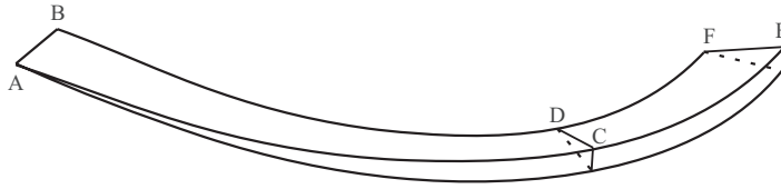
Figure 3 When clothoids are used, the banked track has an edge CD across the track in the turn, through the transition point D .
